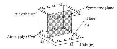
Figure 2.9-3: Indoor model for CFD analysis
