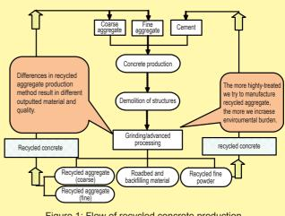
Figure 1: Flow of recycled concrete production
