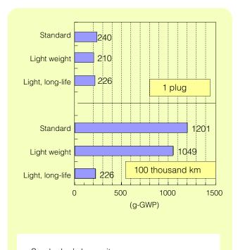
Spark plug's longevity Standard & lightweight: 20 thousand km Light & long- life: 100 thousand km
